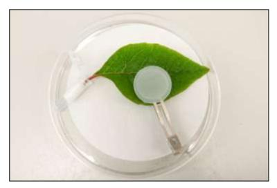
**Figure 2.** *Bemisia tabaci* adults exposed to chemically treated leaf surface in Petri dish (adult whitefly placed on underside of leaf).
